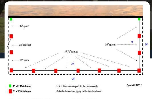
Walls are 8' tall with an 18" kickplate. Single outswing door quoted. Insulated roof is 3" thick
